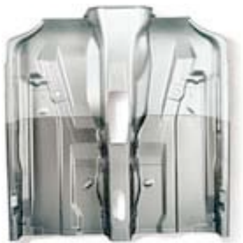
Figure 52: Characteristic picture of a tailor welded blank application
